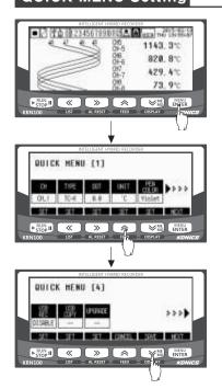
Press the NEW key once in RUN mode and it enters to QUICK MENU. QUICK MENU consists of usually used parameters for quickly parameter setting.
